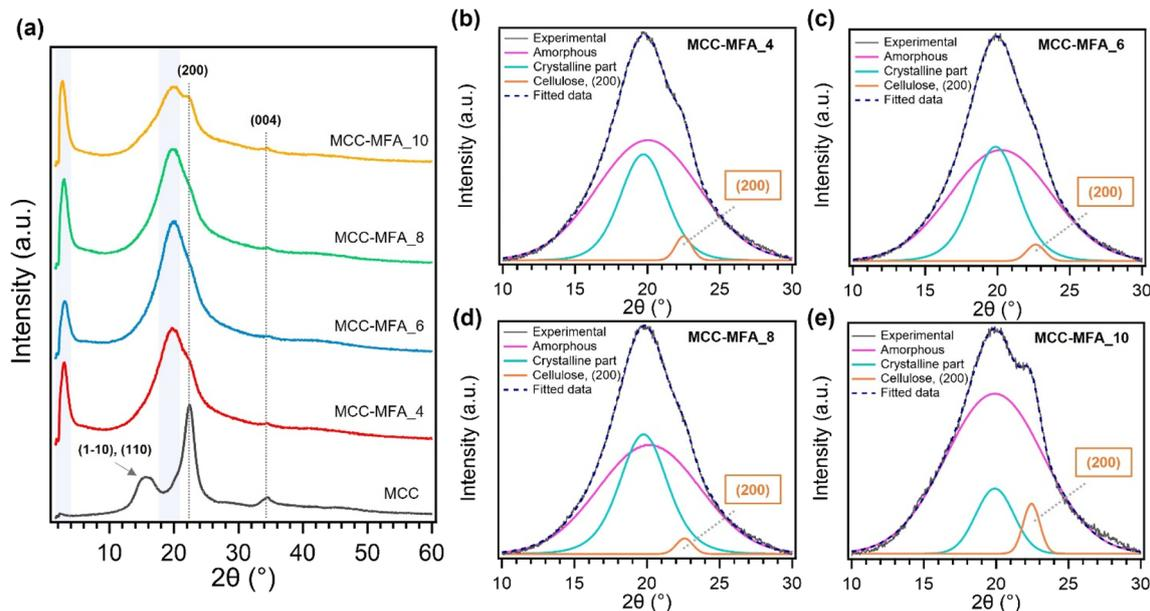
Fig. 3 (a) XRD profiles of MCC and MCC-MFA samples; (b)–(e) deconvoluted peaks superimposed on the experimental curves for MCC-MFA samples.
