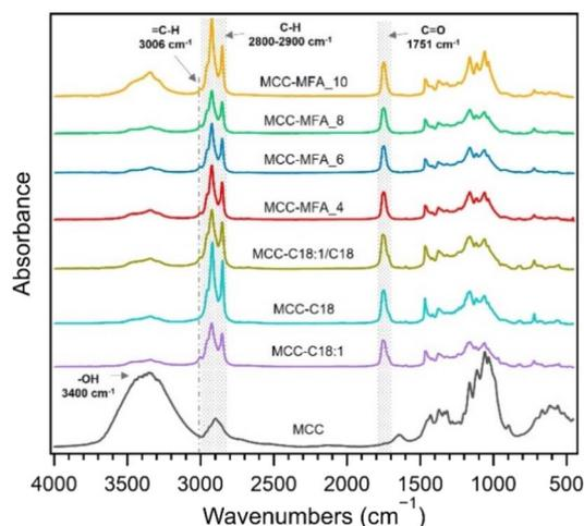
Fig. 1 FT-IR spectra of synthesized cellulose esters.
