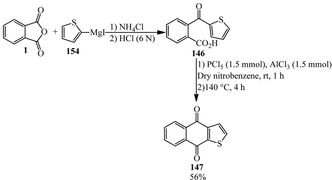
Scheme 54 Reaction of PA and 2-thenoylmagnesium iodide.
