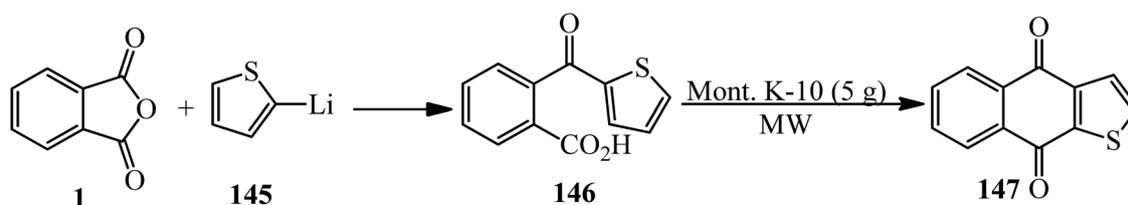
Scheme 51 Synthesis of thieno[2,3-b]-[1,4]-naphthoquinone.
