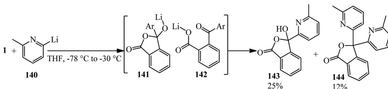
Scheme 50 Addition of pyridinyl lithium to PA.
