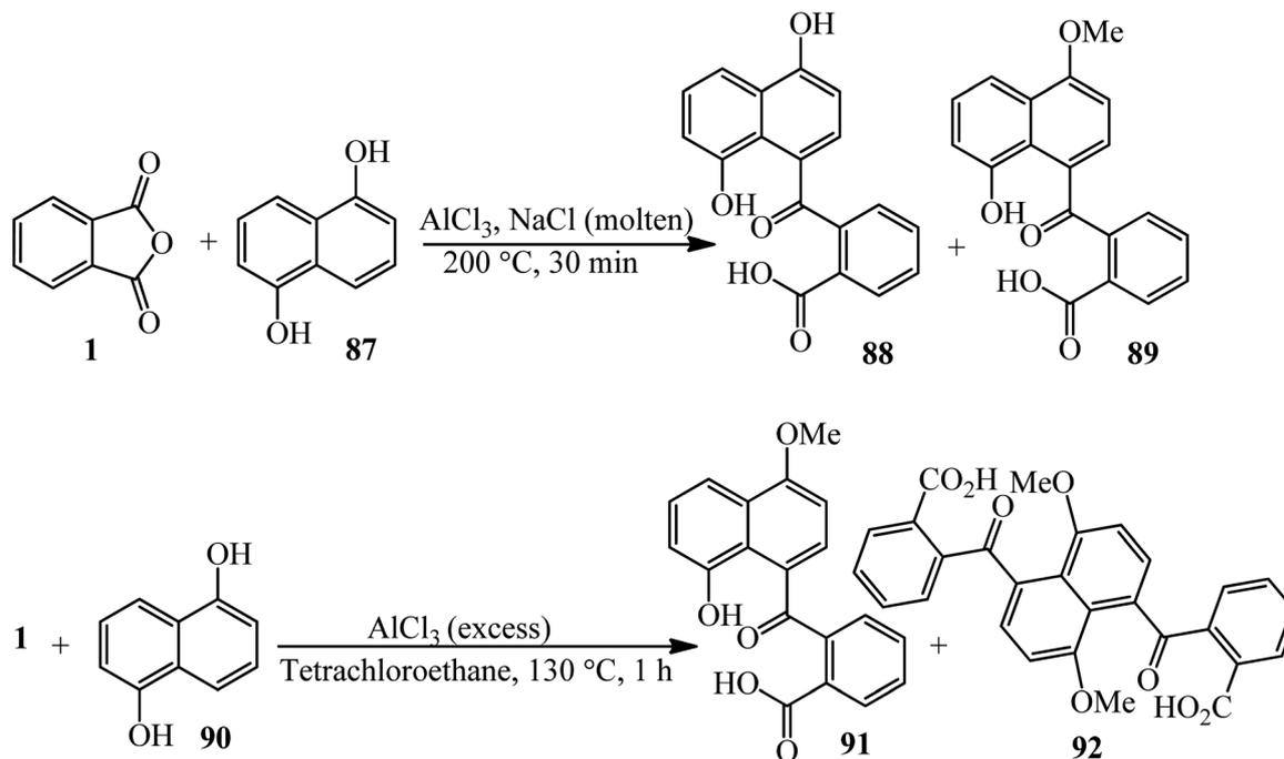
Scheme 34 The Friedel–Crafts reaction of 1,5-dihydroxynaphthalene and 1,5-dimethoxynaphthalene with PA.
