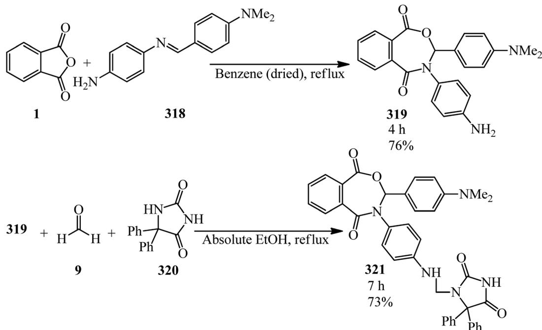
Scheme 120 3-(4-(Dimethylamino)phenyl)-4-(4-(((2,4-dioxo-5,5-diphenylimidazolidin-1-yl)methyl)amino)phenyl)-3,4-dihydrobenzo[e][1,3]xazepane-1,5-dione preparation.
