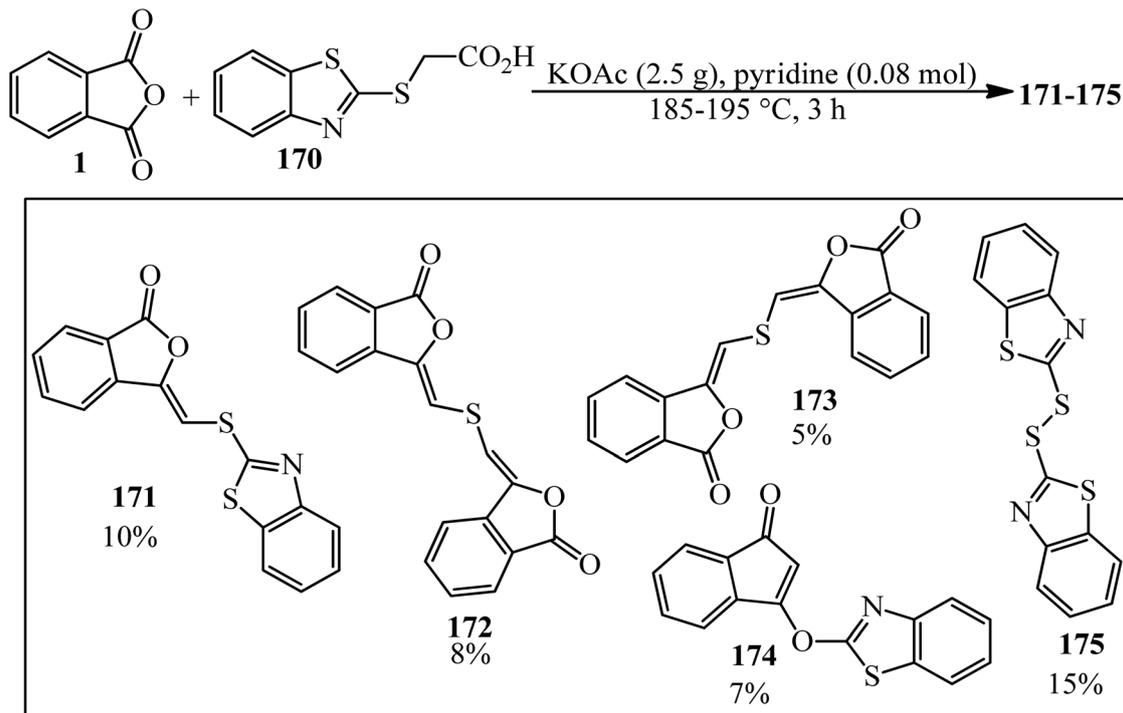
Scheme 65 Reaction of 2-benzothiazolylthioethanoic acid with PA.
