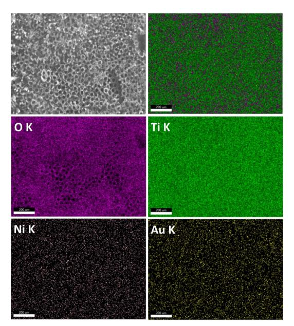
Fig. 5 The EDS elemental mapping of Au<sub>30</sub>/Ni<sub>20</sub>/TiO<sub>2</sub>NTs.
