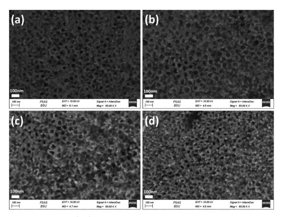
Fig. 4 FESEM images of the top-view of  $Au_y/Ni_{20}/TiO_2NTs$  photoanodes synthesised by different time intervals of photodeposition (a) 15 min, (b) 30 min, (c) 60 min and (d) 120 min.
