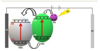
Fig. 13 The proposed mechanism for charge transfer in  ${\rm Au_y/Ni_{20}/TiO_2NTs}$  photoanodes during PEC.
