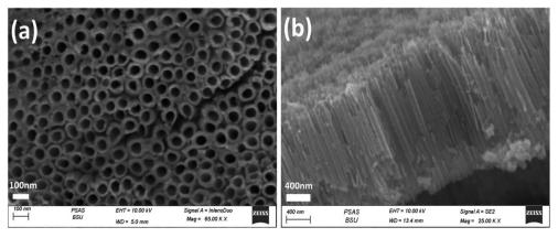
Fig. 2 Top-view (a) and side-view (b) FESEM images of TiO<sub>2</sub>NTs photoanode.
