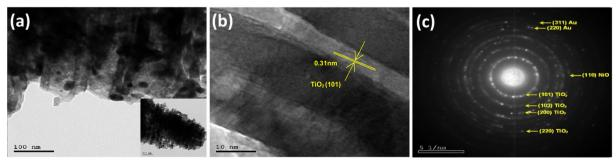
Fig. 6 (a and b) HRTEM images of  $Au_{30}/Ni_{20}/TiO_2NTs$  and (c) SAED patterns of photoanode.
