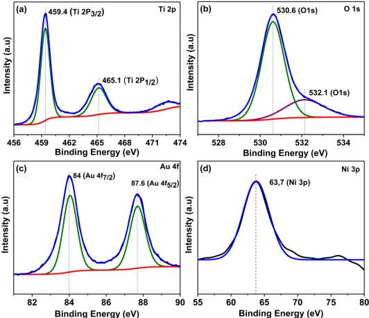
Fig. 8 XPS spectra for Au<sub>30</sub>/Ni<sub>20</sub>/TiO<sub>2</sub>NTs photoelectrode (a) Ti 2p, (b) O 1s, (c) Au 4f and (d) Ni 3p.
