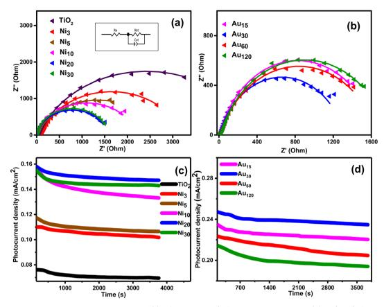
Fig. 12 Electrochemical impedance spectroscopy plot of (a)  $TiO_2NTs$  and  $Ni_x/TiO_2NTs$  photoanodes, and (b)  $Au_y/Ni_{20}/TiO_2NTs$  photoanodes. The proposed equivalent circuit (inset (a)). The stability measurement at 1.0 V for 1 h of (c)  $TiO_2NTs$  and  $Ni_x/TiO_2NTs$  photoanodes, and (d)  $Au_y/Ni_{20}/TiO_2NTs$  photoanodes.
