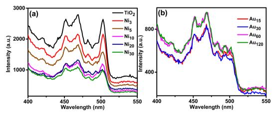
Fig. 10 PL spectra of (a)  $TiO_2NTs$  and  $Ni_x/TiO_2NTs$  photoanodes, and (b)  $Au_y/Ni_{20}/TiO_2NTs$  photoanodes.
