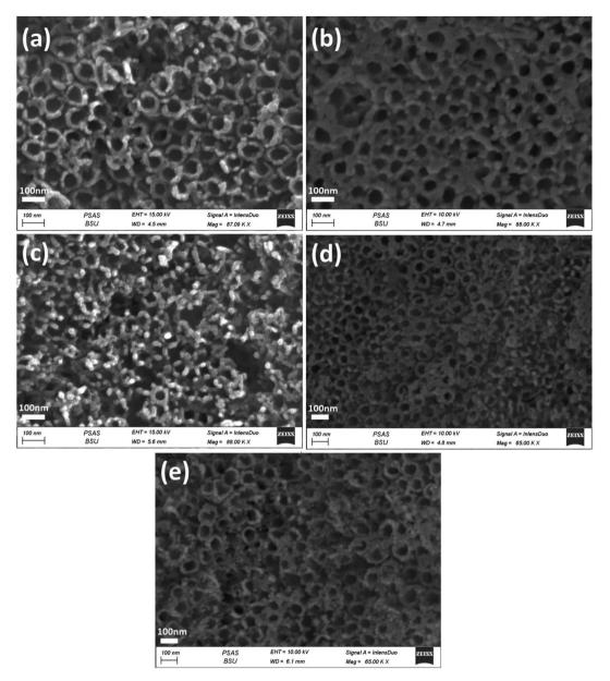
Fig. 3 FESEM images of the top-view of  $Ni_x/TiO_2NTs$  photoanodes synthesised by different electrodeposition cycles (a) 3 cycles, (b) 5 cycles, (c) 10 cycles, (d) 20 cycles and (e) 30 cycles.
