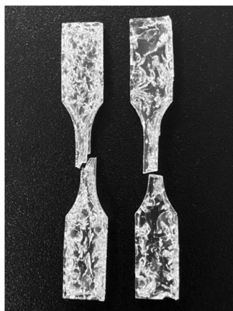
Fig. 10 Physical changes in PLA-PETA-PO resulting from hydrolytic degradation after 280 days.
