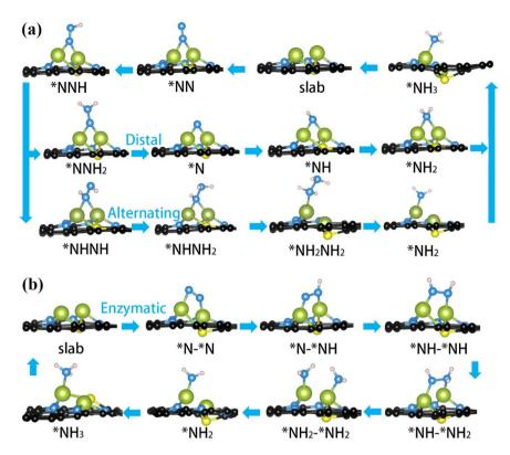
Fig. 2 Optimized structures of every intermediate adsorbed on Fe<sub>2</sub>@SN<sub>4</sub> surface for NRR along distal and alternating pathways with (a) end-on configuration and enzymatic pathway with (b) side-on configuration.
