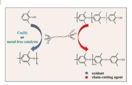
Chemical and physical properties of low-molecular-weight poly(2,6-dimethyl-1,4-phenylene oxide) (LMW-PPO) synthesized by peroxydisulfate and metal/non-metal catalysts
