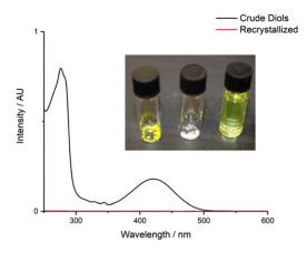
Fig. 6 UV-vis absorption spectra of the crude and recrystallized diol mixture from depolymerization. Inset images from left to right show the crude mixture, the recrystallized trans-cyclohexane-1,2-diol, and the supernatant.
