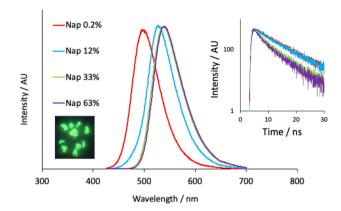
Fig. 4 Solid state emission spectra of Nap-PA-CHO ( $\lambda_{\rm ex}=410$  nm) at different dopant levels. Inset: the corresponding decay profiles ( $\lambda_{\rm ex}=295$  nm) for the different materials (fits yielding lifetimes of 8.0, 7.9, 6.8 (80% weighting) and 2.6% (20% weighting), 7.3 (71% weighting) and 2.4 ns (29% weighting) for Nap dopant levels of 0.2%, 12%, 33% and 63%, respectively).
