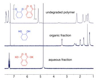
Fig. 5 <sup>1</sup>H NMR spectra (300 MHz) of Nap-PA-CHO and crude organic and aqueous fractions after depolymerization with potassium hydroxide. No signals for the chromophore were observed in the spectra owing to the low concentration (0.2 mol%).
