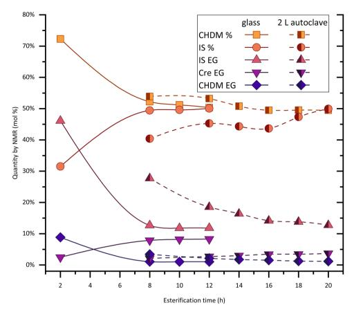
Fig. 7 Scale-up (trans)esterification reaction for PICT in 2-liter autoclave (half-painted symbols) with 0.3 equivalent of cresol compared with small-scale reaction in 100 ml glass reactor (filled symbols) with 0.6 equivalent of cresol. No data on this graph regarding the vacuum steps. Lines/dashed lines are only meant to help with visualization.
