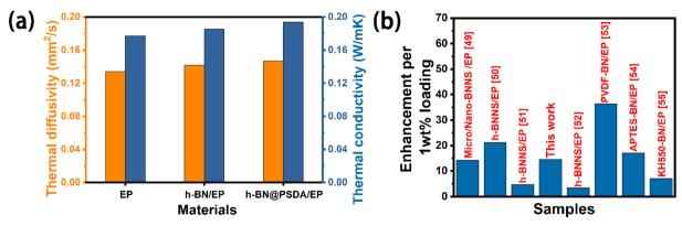
Fig. 5 (a) Thermal diffusivity and thermal conductivities of EPs, h-BN/EPs and h-BN@PSDA/EPs, respectively. (b) Comparison of the enhancement efficiency of the thermal conductivity of the EP composites per 1 wt% h-BN@PSDA fillers
