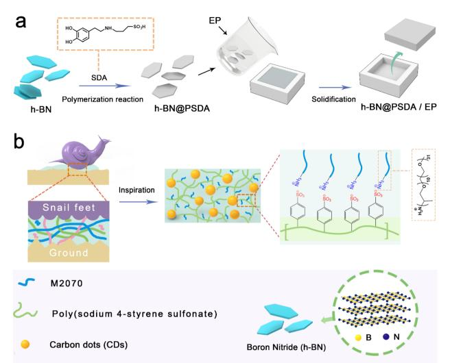
Fig. 1 (a) Synthesis process of h-BN@PSDA and h-BN@PSDA/EPs; (b) schematic diagram of a 3D polymer network on the surface of a solventfree carbon dot nanofluid prepared inspired by the mucus lubrication system of a snail.
