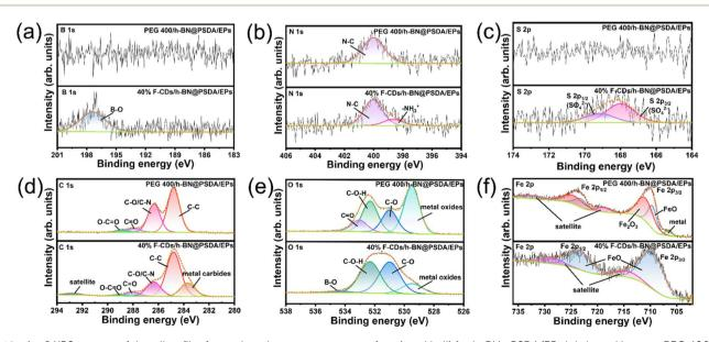
Fig. 10 (a-f) XPS spectra of the tribo-film formed on the worn counter surface (steel ball) for h-BN@PSDA/EPs lubricated by pure PEG 400 and 40 wt% F-CDs in PEG 400.
