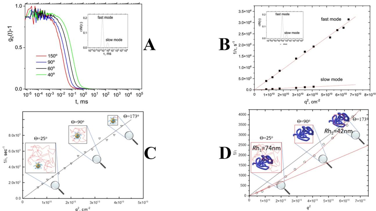
Fig. 6 Angle dependence of the correlation function; inset: bimodal distribution function (A);  $q^2$  dependence of inverse correlation/decay time for fast and slow modes obtained from a distribution function (B);  $q^2$  dependence of inverse correlation/decay time for small nanoparticles (C);  $q^2$  dependence of inverse correlation/decay time for large nanoparticles. The red solid line represents the fitting with eqn (4) (D).
