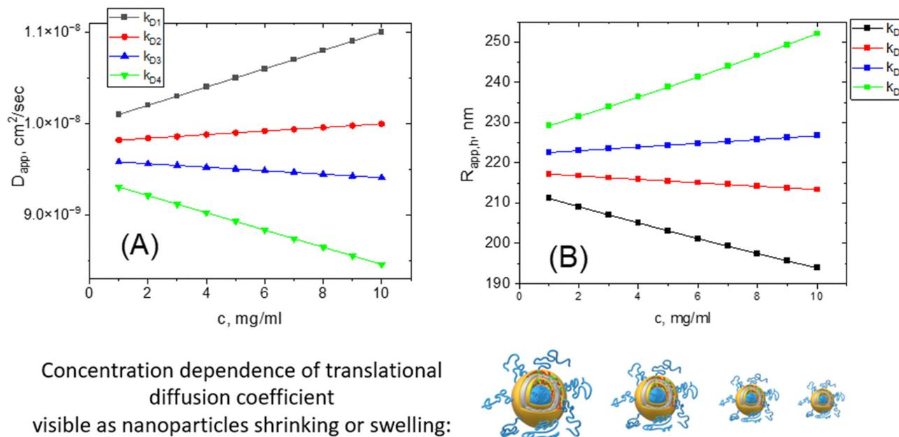
Fig. 7 The example of concentration dependence of apparent translational diffusion coefficient for different  $k_D$  values (A); the concentration dependence of apparent hydrodynamic radii calculated from  $D_t$  (B).
