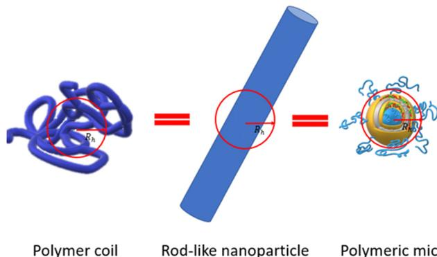
**Fig. 5** Red circle represents hydrodynamic size as seen by DLS. Three different nano-objects with highly distinctive morphologies such as a polymer coil, rod-like nanoparticle, and a polymeric micelle have the same hydrodynamic size. This cartoon represents the fact that DLS is a “blind” method that provides the value of a diffusion coefficient converted later to hydrodynamic size. The mismatch depends on architecture and draining of the nanoparticles.
