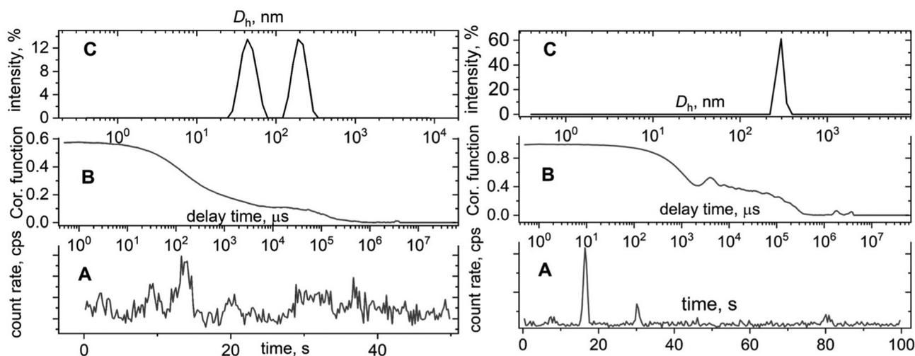
**Fig. 2** Example of poor-quality measurements: typical count rate (A), correlation function (B), and  $D_h$  distribution function (C) for samples containing dust or large aggregates (left); and for even the worst case of system sedimentation (right).
