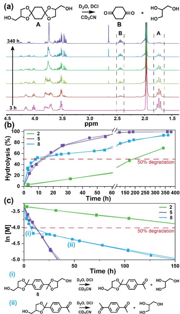
**Fig. 5** (a) Time-resolved <sup>1</sup>H-NMR spectra for the hydrolysis of intermediate 2 by monitoring the integration of (A) ketal and (B) ketone peaks over 340 h at ambient temperature (20 °C). (b) Hydrolysis kinetics plotted for 2, 5, and 8 vs. time. (c) Semilogarithmic kinetic plot for the hydrolysis of 2, 5, and 8. Two kinetic regimes and the associated structures for hydrolysis of 8 are indicated by (i) and (ii).
