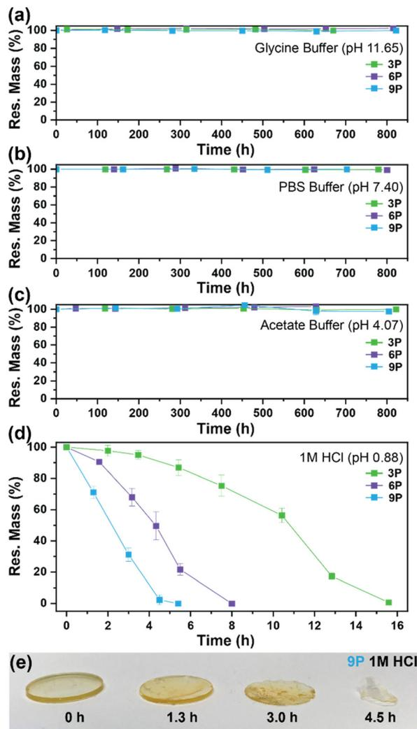
**Fig. 6** Mass-loss degradation versus time for 3P, 6P, and 9P in (a) glycine buffer (pH 11.65), (b) PBS buffer (pH 7.40), (c) acetate buffer (pH 4.07), and (d) 1 M HCl (pH 0.88). Experiments were conducted at ambient lab temperature (20 °C). (e) Snapshot photos of 9P disks pulled from 1 M HCl at various time intervals to illustrate surface erosion.
