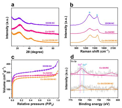
Fig. 3 (a) XRD patterns, (b) Raman spectra, and (c) N₂ adsorption-desorption isotherms of Co-SA/3DOM-NC, Co-SA/NC, and 3DOM-NC. (d) Highresolution Co 2p XPS spectra of Co-SA/3DOM-NC and Co-SA/NC.
