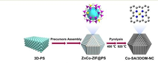
Fig. 1 Schematic illustration of the fabrication of Co-SA/3DOM-NC
