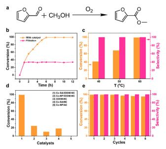
Fig. 6 (a) Catalytic oxidative esterification of FFA to methyl 2-furoate. (b) Activity profiles for the oxidation esterification of FFA over Co-SA/ 3DOM-NC. (c) The effects of temperature on the FFA conversion and methyl 2-furoate selectivity over Co-SA/3DOM-NC. (d) comparison of the FFA conversion between Co-SA/3DOM-NC and other catalysts. (e) Reusability tests of Co-SA/3DOM-NC for the oxidative esterification of FFA.
