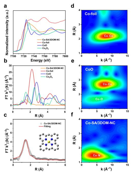
Fig. 4 (a) XANES spectra and (b) Fourier-transform EXAFS spectra of Co-SA/3DOM-NC, Co foil, CoO, and Co₃O₄. (c) Fourier-transform EXAFS fitting curves of Co K-edge for Co-SA/3DOM-NC (inset: a proposed structural model of Co-SA/3DOM-NC). Wavelet-transformed contour plots of Co in (d) Co foil, (e) CoO, and (f) Co-SA/3DOM-NC.
