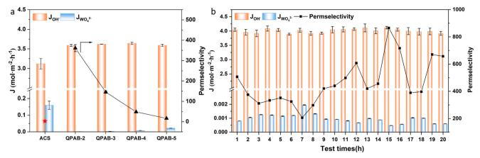
Fig. 7 (a) Anion fluxes and permselectivities of the Neosepta ACS and QPAB-x membranes in a NaOH/Na<sub>2</sub>WO<sub>4</sub> system at a current density of 10 mA cm<sup>-2</sup>; (b) operational stability of the QPAB-2 membrane for continuous ion selectivity.
