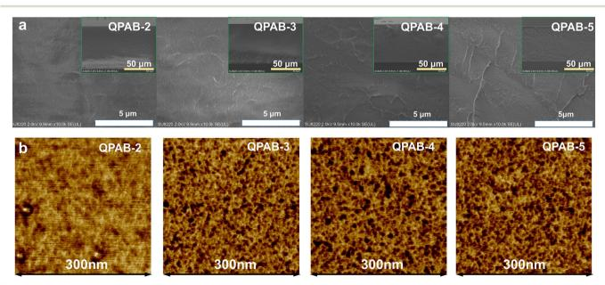
Fig. 2 Morphology features of QPAB-x membranes. (a) SEM cross-section images of QPAB-x membranes; (b) AFM phase images of QPAB-x membranes
