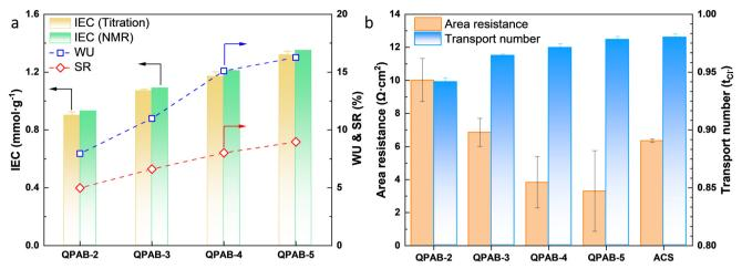
Fig. 3 Physical and electrochemical characteristics of QPAB-x and Neosepta ACS membranes. (a) IEC, WU and SR of QPAB-x membranes; (b) area resistance and transport number of QPAB-x and Neosepta ACS membranes.
