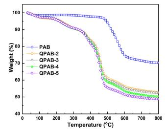
Fig. 4 TGA thermograms of PAB and QPAB-x membranes in a N<sub>2</sub> atmosphere.
