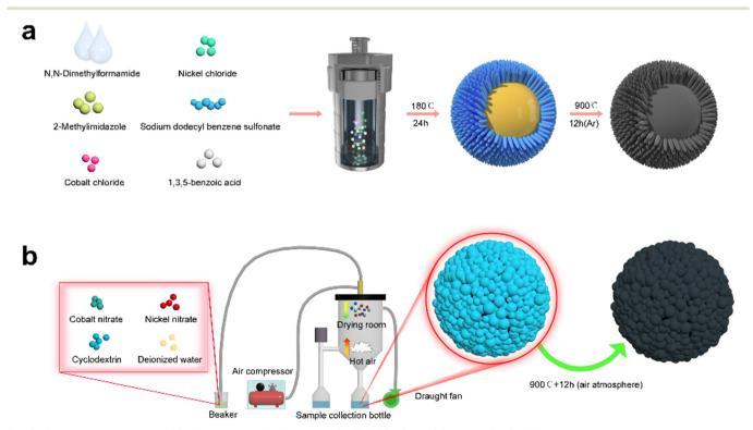
Fig. 6 Synthesis process of the (a) yolk-shell urchin-like porous Co<sub>3</sub>O<sub>4</sub>/NiO@C and (b) porous Co<sub>3</sub>O<sub>4</sub>/NiO microspheres.
