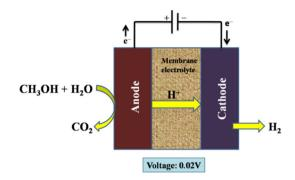
Fig. 24 Electrolysis using organic fuel methanol.
