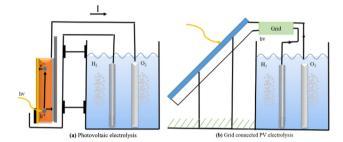
Fig. 18 (a) Photovoltaic electrolysis. (b) Grid-connected PV electrolysis.
