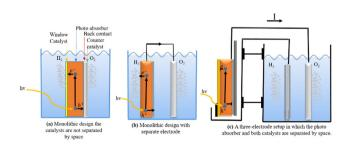
Fig. 17 (a) Monolithic design where the catalysts are not separated by space. (b) Monolithic design with separated electrode. (c) A three-electrode setup in which the photoabsorber and both catalysts are separated by space.
