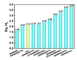
**Fig. 9** Dehydrogenation yields of EDB supported by imidazolium-based ILs. Reproduced with permission.<sup>67</sup> Copyright 2013, Elsevier.
