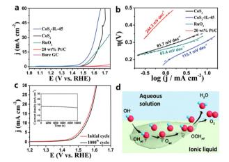
Fig. 3 (a) OER LSV curves of the bare GC electrode, commercial 20 wt% Pt/C, CoS<sub>2</sub> and IL-modified CoS<sub>2</sub> and (b) the derived Tafel plots. (c) OER LSV curves of IL-modified CoS<sub>2</sub> before and after 1000 CV tests. (d) Schematic illustration of the oxidation of water. Reproduced with permission. 46 Copyright 2018, the Royal Society of Chemistry.
