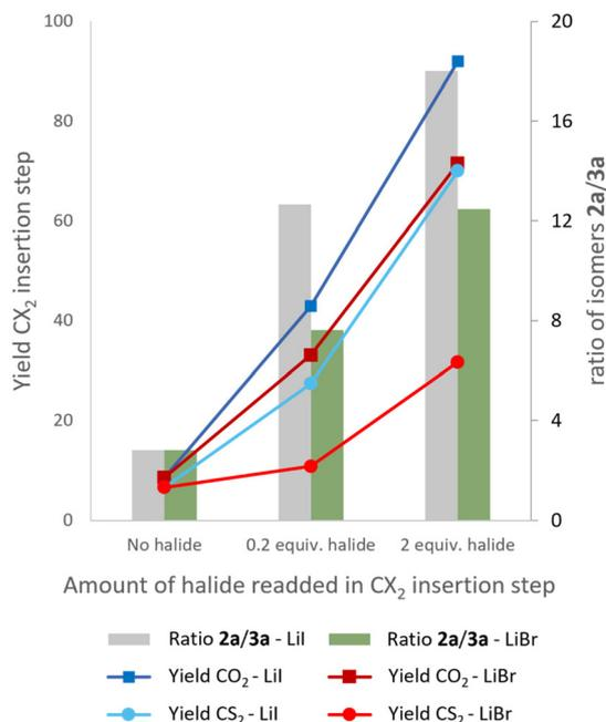
**Fig. 1** Control experiments where the influence of the halide is studied regarding the yield of the CX<sub>2</sub> insertion step towards products **2a** or **4a** (curves, left y-axis) and the distribution of isomers **2a** and **3a** (bars, right y-axis) using <sup>1</sup>H-NMR. See ESI for more experimental details.†
