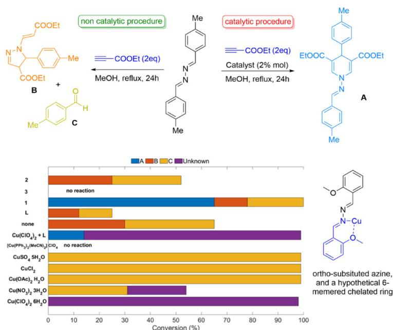
**Fig. 4** Control experiments for the synthesis of dihydropyridines. **1** corresponds to  $[\text{Cu}^{\text{II}}(\text{L1})_2(\text{MeCN})_2] \cdot 2(\text{ClO}_4) \cdot \text{MeCN}$ , **2** to  $[\text{Zn}^{\text{II}}(\text{L1})_2(\text{H}_2\text{O})_2] \cdot 2(\text{ClO}_4) \cdot 2\text{MeCN}$  and **3** to  $[\text{Cu}^{\text{II}}(\text{L1})(\text{NO}_3)_2] \cdot \text{MeCN}$  (see Table 2 for more info).
