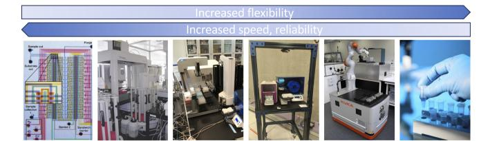
Fig. 2 Automation systems span a continuum of flexibility, speed, and reliability, from the integrated (e.g., as shown here, a microfluidic laboratory) to the fixed (e.g., Adam¹), flexible (e.g., a bio workcell at Argonne), reconfigurable (e.g., a "cart" in Argonne's RPL), mobile (e.g., Liverpool's mobile robotic chemist<sup>6</sup>), and manual
