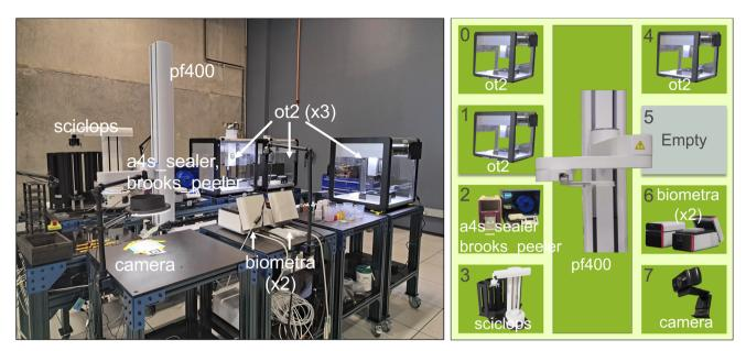
Fig. 8 A photo (left) and schematic (right) of the RPL workcell, comprising eight carts, #0-#7, plus a central pf400 plate mover for transferring sample trays among carts. Modules are labeled with the nicknames in Table 2. Cart #5 is empty, and carts #2 and #6 each contain two modules.
