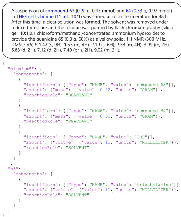
Fig. 8 The organic synthesis parser interface. The top box shows text describing an organic reaction ( https://open-reaction-database.org/client/id/ord-1f99b308e17340cb8e0e3080c270fd08 ), which the finetuned LLM converts into structured JSON (bottom). A demo application can be found at https://qai222.github.io/LLM_organic_synthesis/ .
