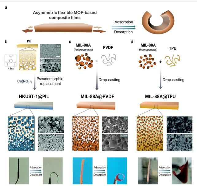
Fig. 3 Schematic of the folding mechanism in asymmetric, flexible-MOF, composite films (a). Schematic of the syntheses, and photographs illustrating the reversible bending, of asymmetric HKKUST-1@PIL (b), MIL-88A@PVDF (c), MIL-88A@TPU (d) (scale bars = 2 µm). Adapted, with permission, from ref. 30, 38 and 40.
