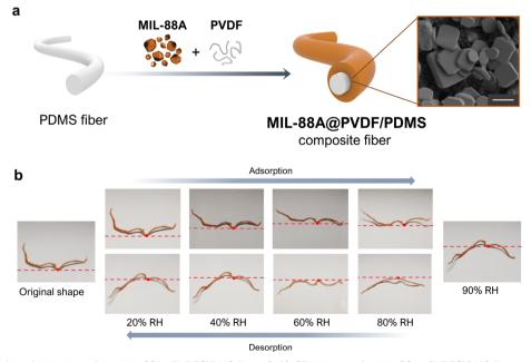
Fig. 6 (a) Schematic of the fabrication of the MIL-88A@PVDF/PDMS fibres (left). SEM image of a MIL-88A@PVDF/PDMS fibre, revealing the embedding of MIL-88A within the PVDF polymer matrix (right). Scale bar (1 µm). (b) Photographs of the deformation of MIL-88A@PVDF/PDMS fibre upon exposure to different levels of relative humidity (RH): from 20% up to 90% (adsorption), and from 90% back down to 20% (desorption). Adapted, with permission, from ref. 54.
