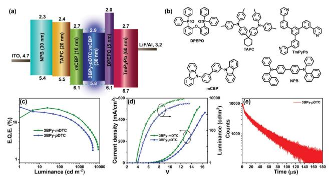
Fig. 3 OLED device fabrication: (a) device architecture, (b) molecular structure of the materials used in the device, (c) luminance vs. EQE, (d) current density and luminance vs. driving voltage and (e) transient electroluminescence characteristics of the **3BPy-pDTC** device.
