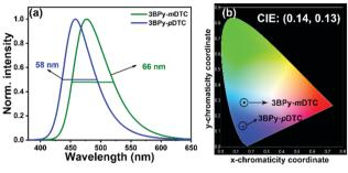
Fig. 4 Blue OLED device based on TADF emitters: (a) electroluminescence (EL) spectra and (b) CIE chromaticity diagram of 3BPy-pDTC and 3BPy-mDTC depicting the color purity based on the narrow FWHM and CIE coordinates towards pure blue emission
