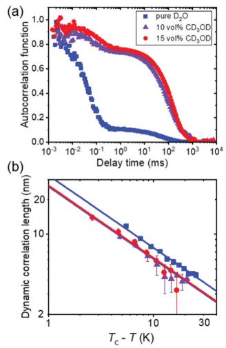
**Fig. 4** Results from DLS on a semidilute solution of PNIPAM (9 wt%) in mixtures of  $D_2O$  and  $CD_3OD$  having the  $CD_3OD$  volume fractions given in (a). <sup>49</sup> (a) Representative normalized intensity autocorrelation functions at 22 °C. (b) Dynamic correlation length from the fast mode of all solutions vs.  $T_c-T$  in a double-logarithmic representation, where  $T_c$  is the critical temperature. Same symbols as in (a). The lines have a slope of -0.63.
