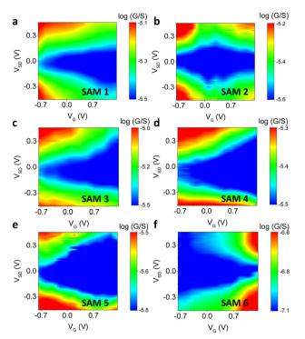
Fig. 4 Experimental plots of  $\log G$  vs.  $V_G$  and  $V_{SD}$  for SAMs **1-6** (a-f, respectively)
