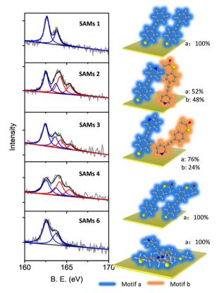
Fig. 2 Comparison of XPS S2p spectra measured for SAMs of molecules 1-4 and 6 (5 showed identical features to 4) (left). Different binding motifs present within the SAMs on Au (right)
