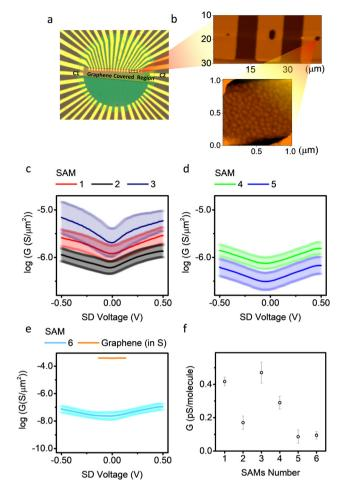
Fig. 3 (a and b) Optical micrographs of a typical micro-well-based device used in this work. (c-e) Conductance G on a log scale vs. applied sourcedrain voltage for SAMs 1-5, and in-plane conductance across graphene. (f) Zero-bias conductance of molecules 1-6.
