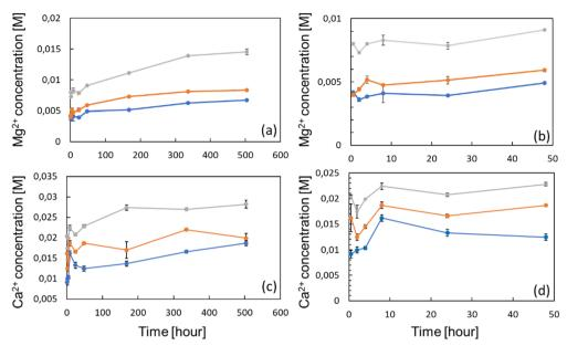
Fig. 3 Global release profiles of  $Mg^{2+}$  ions from FAU zeolites from 0.5 to 504 h (a), and the corresponding profiles of  $Ca^{2+}$  ions (c). Same profiles focused on the first 48 h for (b)  $Mg^{2+}$  ions and (d)  $Ca^{2+}$  ions. Three zeolite concentrations were used, namely 1 wt% (blue), 1.5 wt% (orange), and 3 wt% (gray). The values are represented as mean SD, n = 3.
