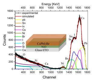
Fig. 3 RBS spectrum with the fitting of multilayer samples, i.e., glass/ITO/ NiO<sub>x</sub>/CsPbl<sub>2</sub>Br, excited from the IHP side, along with deconvolution of the elemental spectra
