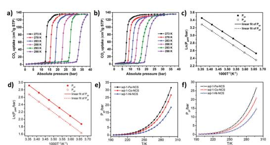
Fig. 3 High-pressure CO<sub>2</sub> sorption isotherms of (a) sql-1-Fe-NCS and (b) sql-1-Ni-NCS. The linear fit of gate sorption pressure (LnP) and temperature  $(1000 \text{ T}^{-1})$  using the Clausius-Clapeyron equation for (c) **sql-1-Fe-NCS** and (d) **sql-1-Ni-NCS**. (e) Calculated  $P_{\text{qa}}$  and (f)  $P_{\text{qd}}$  for **sql-1-M-NCS** (M = Fe,
