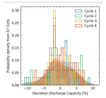
Fig. 3 Distribution of discharge capacity deviation from the median for the respective cycle. Bootstrapping results in a mean of 4.16 (4.12, 4.20) mA h with the values in brackets being the 90% confidence interval, the standard variation from bootstrapping is 0.144 mA h. In the fourth cycle 90% of the cells are within a 10% error range and 60% are within a 5.9% error range.
