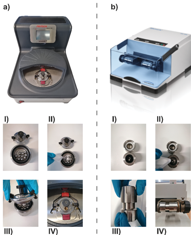
Fig. 1 Upper part: Examples of (a) a planetary ball mill (Fritsch planetary ball mill P7) and (b) a vibrational ball mill (Retsch mixer mill MM400). Lower part: Procedure of milling jar filling for (left) a planetary ball mill and (right) a vibrational ball mill. (I) The empty milling jars are equipped with a seal and milling balls. (II) The mill charge is added to the jar. (III) Milling jars are properly closed. (IV) Implementation of the milling jars in the respective ball mill.
