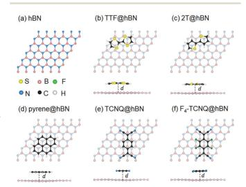
(a) A  $6 \times 6$  supercell of hBN monolayer; top and side views of the hybrid interfaces formed by (b) tetrathiafulvalene (TTF), (c) bithiophene (2T), (d) pyrene, (e) tetracyanoquinodimethane (TCNQ), and (f) fluorinated TCNQ (F<sub>4</sub>-TCNQ) adsorbates
