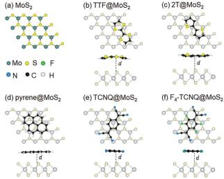
Fig. 2 (a) A  $4 \times 4$  supercell of MoS<sub>2</sub> monolayer; top and side views of hybrid interfaces formed by (b) tetrathiafulvalene (TTF), (c) bithiophene (2T), (d) pyrene, (e) tetracyanoguinodimethane (TCNQ) and (f) fluorinated TCNQ (F<sub>4</sub>-TCNQ) adsorbates.
