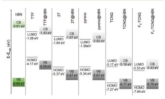
Fig. 3 Energy level alignment computed for the hBN-based hybrid interfaces using the HSE06 + rVV10 hybrid functional
