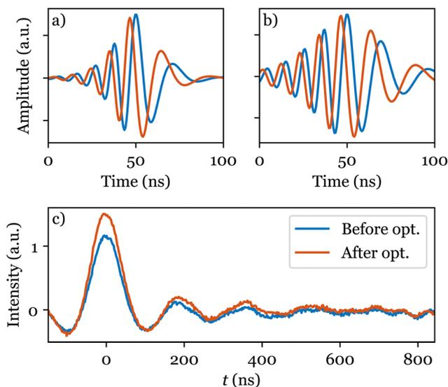
Fig. 3 Cartesian representation of the HS pump pulse in a 4-pulse DEER experiment, (a) before ( $\beta = 10$ ), and (b) after ( $\beta = 6$ ) optimisation, with (c) corresponding full DEER traces for bisnitroxide (Scheme 1).
