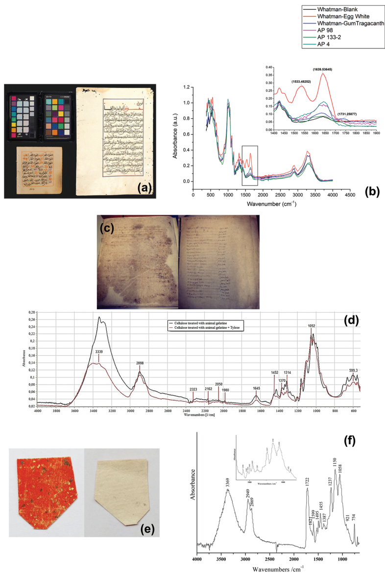
Fig. 6 (a) Two objects in the historic reference material collection at UCL Institute for Sustainable Heritage and (b) the proteinaceous coatings have peaks of amide group bonds at 1533 and 1639 \text{cm}^{-1} in ATR-FTIR spectra. Reproduced with permission, 117 copyright (2016) Springer Nature. (c) Paper documents from Camerino. (d) ATR-FTIR spectra of cellulose samples show that the restoration materials Tylose may make gelatine spectral bands at 1540 and 1645 \text{cm}^{-1} less visible. Reproduced with permission, 119 copyright (2020) Elsevier Masson SAS. (e) Lajian paper sample with Au/Ag flakes and upper orange-red layer (left) and backing layer (right), coated with (f) Chinese insect wax which has absorbance of carboxyl group at 1722 \text{cm}^{-1} . Reproduced with permission, 121 copyright (2019) Springer Nature.
