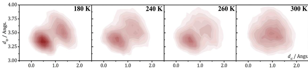
Fig. 19 2D-PDF's associated with the interplanar distance ( $d_{ip}$ ) and the relative latitudinal slippage ( $d_{sl}$ ) between adjacent NCBDTA radicals, as obtained from AIMD trajectories run at 180, 240, 260 and 300 K. Figure reprinted with permission of ref. 112.
