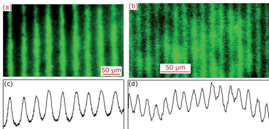
Fig. 2 Fluorescence microscope images and corresponding cross-sectional profiles of hydrogel films patterned using the IL set-up comprising FB with  $\alpha$  of (a and c) 179 deg and (b and d) 177 deg.
