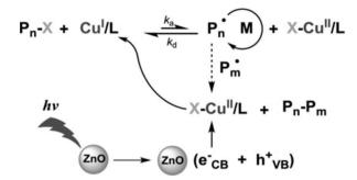
Fig. 2 Proposed mechanism of ATRP using ZnO as the photocatalyst. Reproduced from ref. 66 with permission from Wiley-VCH Verlag GmbH & Co. KGaA, Weinheim, copyright 2014.
