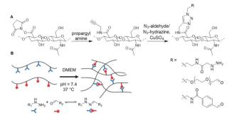
**Fig. 16** Crosslinking of HA with adjustable crosslinks. A. Propargylamine was conjugated to NHS-activated HA. Aldehyde and hydrazone functionalities were introduced *via* CuAAC chemistry. B. Crosslinking of HA *via* dynamic hydrazone bond formation. Adapted and reprinted from ref. 111 with permission from Elsevier, copyright (2018).
