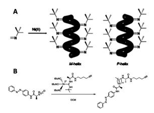
Fig. 31 A. Formation of stable helix by polymerizing *tert*-butylisocyanide with a nickel(III) catalyst. Reproduced from ref. 214 with permission from the Royal Society of Chemistry, copyright (2011). B. Isocyanide polymerization with an alkyne-modified nickel(III) catalyst to introduce an alkyne handle on the polymer chain-end. Reprinted from ref. 225 with permission from John Wiley and Sons, copyright (1969).
