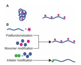
Fig. 1 A. Schematic representation of the difference between flexible (left) and semiflexible (right) polymer scaffolds. The more stretched chain conformation of the latter provides a much better access to substituents grafted to the polymer. B. Schematic overview of the different strategies for the introduction of substituents on semiflexible polymer scaffolds as discussed in this review.
