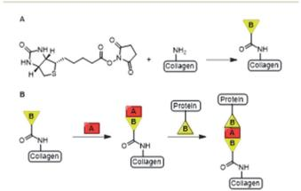
Fig. 3 A. The bridged avidin and biotin procedure for conjugation of EGF and HBGF2 to collagen. NHS-functionalized biotin was conjugated to collagen, EGF and HBGF2 via amide bond formation. Reprinted from ref. 16 with permission from Elsevier, copyright (1989). B. Avidin (A) was used a bridge between two biotinylated (B) compounds, the scaffold and biotinylated growth factors EGF or HBGF2. Reprinted from ref. 18 with permission from John Wiley and Sons, Copyright (1969).
