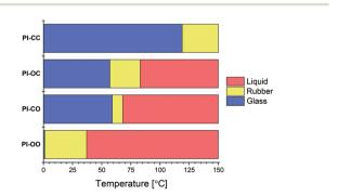
**Fig. 4** Visual representation of the glass (blue), rubber (yellow) and liquid (red) phases of the **PI-XX** materials as a function of the temperature.
