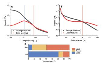
Fig. 2 Representative temperature sweep curves of (A) PI-C and (B) PI-O, where the vertical blue line indicates the glass-rubber transition and the vertical red line indicates the rubber-liquid transition. (C) Visual representation of the glass (blue), rubber (yellow) and liquid (red) phases of PI-O (top) and PI-C (bottom) as a function of the temperature.
