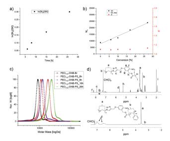
Fig. 1 Synthesis and characterization of PEO-ONB-b-PS diblock copolymers. (a) Logarithmic plot of monomer consumption versus time. (b) Linear relation of molecular weight and polymer dispersity versus conversion. (c) GPC traces during the polymerization of PEO<sub>113</sub>-ONB-b-PS at varying t. (d) <sup>1</sup>H NMR of PEO<sub>113</sub>-ONB-Br and PEO<sub>113</sub>-ONB-b-PS<sub>90</sub>.
