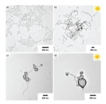
Fig. 6 Morphologies of PEO<sub>113</sub>-ONB-b PS $_x$  BCPs in water. TEM of P2 cylinder micelles at c=0.1 mg mL $^{-1}$  before irradiation (a) and after irradiation (b). TEM of P3 vesicles at c=0.1 mg mL $^{-1}$  before irradiation (c) and after irradiation (d).
