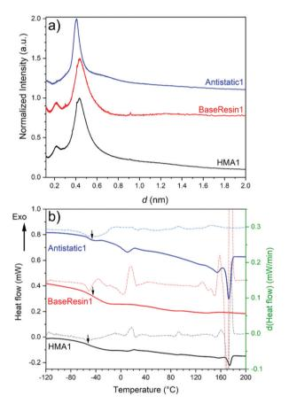
Fig. 4 (a) X-ray diffractograms (see Table S11 $\dagger$  for peak position, d-spacing, and intensity) and (b) DSC (solid line) and first derivative (dotted line) of Antistatic1 (blue), BaseResin1 (red), and HMA1 (black). Graphs were offset for readability.
