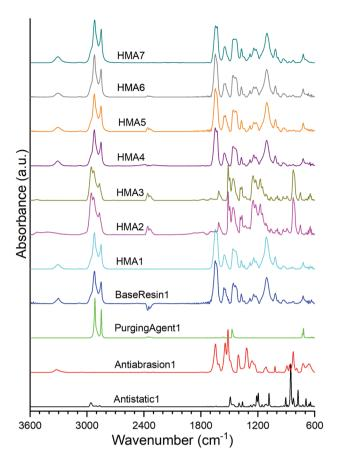
Fig. 1 ATR-FTIR spectra of HMA samples, BaseResin1, PurgingAgent1, Antiabrasion1, and Antistatic1. The full band assignment is given in Table S1. $\dagger$
