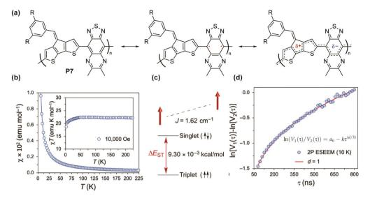
Fig. 10 (a) Closed-shell and open-shell resonance forms of P7; (b)  $\gamma - T$  and  $\gamma T - T$  plots obtained by SQUID measurement; (c) energy diagram of singlet and triplet states; (d) two-pulse electron spin echo instantaneous diffusion data. Reproduced from ref. 76 with permission from the American Association for the Advancement of Science.
