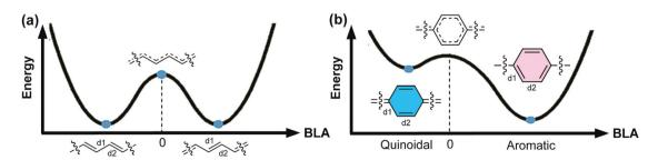
Fig. 1 Energy diagrams of the ground states of the infinite chain of (a) polyacetylene and (b) poly-para-phenylene (PPP) as a function of BLA, which is defined as  $(d_2 - d_1)/2$ . Reproduced (adapted) from ref. 8 with permission from John Wiley and Sons.
