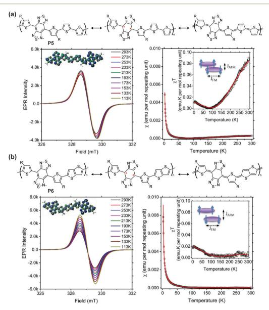
Fig. 9 Closed-shell and open-shell structures of P5 (a) and P6 (b), and their variable-temperature-EPR spectra,  $\chi$ -T and  $\chi$ T-T plots [inset: diagram showing ferromagnetic (FM) and antiferromagnetic (AFM) coupling of spins]. Reproduced from ref. 94 with permission from the American Chemical Society.
