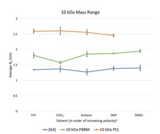
**Fig. 8** Calculated average  $R_h$  values, from DOSY- $^1$ H NMR, for Tetra[G4] Bnz<sub>32</sub>, 10 kDa PCL, and 10 kDa PBBM in all tested solvents.  $^a$ Solvent polarity values from Reichardt were used to determine order of polarity.  $^{39}$
