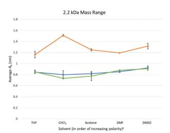
**Fig. 6** Calculated average  $R_{\rm h}$  values, from DOSY- $^{1}$ H NMR, for Tetra[G2] Bnz<sub>8</sub>, 2.2 kDa PCL, and 2.2 kDa PBBM in all tested solvents.  $^{\rm a}$  Solvent polarity values from Reichardt were used to determine order of polarity.  $^{39}$
