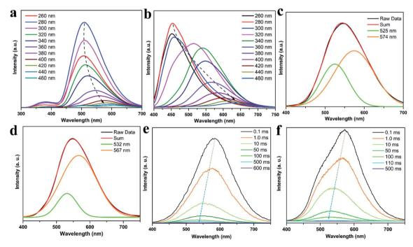
Fig. 6 (a) RTP emission spectra of CDs@IPA and (b) CDs@MA under different excitation wavelengths. (c) The RTP emission spectra of CDs@IPA and (d) CDs@MA at  $\lambda_{ex} = 360$  nm, and the Gaussian fitted by two emission peaks. (e) Time-resolved emission spectra of CDs@IPA and (f) CDs@MA.
