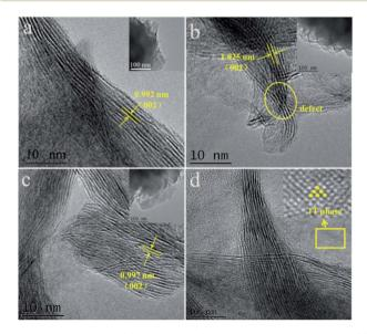
Fig. 4 TEM images of (a)  $220\text{-MoS}_2$ , (b)  $200\text{-MoS}_2$ , (c)  $180\text{-MoS}_2$ , (d) HRTEM images of the in-plane  $1T\text{-MoS}_2$ .
