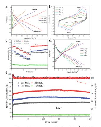
Fig. 6 (a) Charge/discharge curves of  $MoS_2$  at 2 A  $g^{-1}$  with different temperatures, (b) CV curves of  $200\text{-}MoS_2$  at different scan rates, (c) rate performance of  $MoS_2$  at different temperatures, (d) charge—discharge profiles of  $200\text{-}MoS_2$  at the various current densities, (e) cycle performance of  $MoS_2$  at different temperatures.
