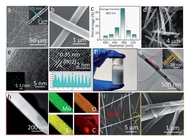
Fig. 1 (a) and (b) SEM images of the AgNF network (inset: SEM image of AgNFs after removing PVA). (c) Diameter histogram of AgNFs. (d) SEM, (e) TEM, and HRTEM images of the as-synthesized MoO<sub>3</sub> nanowires, the inset shows a SAED pattern. (f) Digital image of the MoO<sub>3</sub>/PEDOT:PSS dispersion. (q) TEM, HRTEM, and (h) elemental-mapping images of PEDOT:PSS-glued MoO<sub>3</sub> nanowires. (i) SEM image of the AMP electrode.
