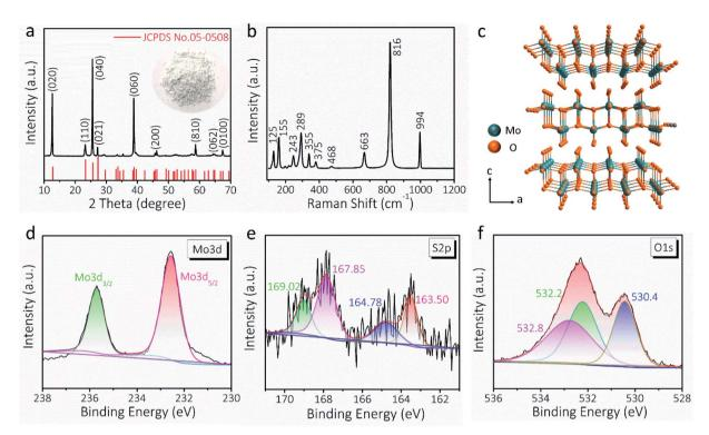
Fig. 2 (a) XRD pattern and (b) Raman spectrum of the as-synthesized  $MoO_3$  nanowires (inset: a digital image of as-synthesized  $MoO_3$  nanowires powder). (c) Schematic diagram of the  $\alpha$ - $MoO_3$  crystal structure. XPS spectra of (d) Mo 3d, (e) S 2p, and (f) O 1s for PEDOT:PSS-glued  $MoO_3$  nanowires.
