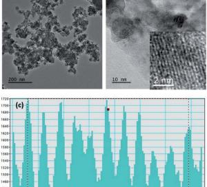
Fig. 1 (a) TEM image, (b) HRTEM image, and (c) intensity profile along the area given in the inset of (b) of the MnO<sub>2</sub> nanostructures.
