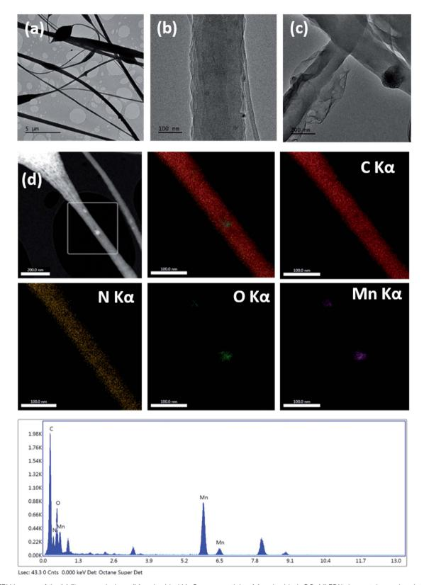
Fig. 4 TEM images of the (a) fiber morphology, (b) embedded MnO<sub>2</sub> nanoparticles, (c) embedded rGO, (d) EDX elemental mapping data and EDX spectrum of the rGOMnPAN fibers.
