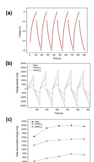
Fig. 8 (a) CCCD cycles in degassed 0.1 M KNO<sub>3</sub> using C-rGOMnPANdeposited graphene sheets as the working electrode, Ag/AgCl as the reference electrode and the Pt sheet as the counter electrode and (b) CDI performance using 100 ppm NaCl, 100 ppm Pb(NO<sub>3</sub>)<sub>2</sub> and 100 ppm Cd(NO<sub>3</sub>)<sub>2</sub> electrolytes; (c) salt removal capacity of the CrGOMnPAN electrode.
