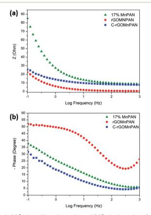
Fig. 6 (a) Bode total impedance plots and (b) Bode phase plots of the 17% MnPAN, 1% rGOMnPAN and C-rGOMnPAN electrodes.
