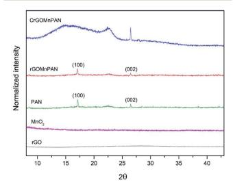
Fig. 2 X-ray diffraction patterns of rGO, the MnO<sub>2</sub> nanoparticles, PAN fibers, 1% rGOMnPAN fibers and C-rGOMnPAN fibers.
