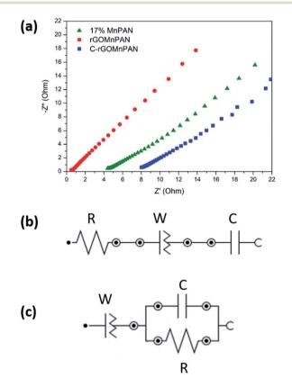
Fig. 7 (a) Nyquist plots of the 17% MnPAN, 1% rGOMnPAN and C-rGOMnPAN electrodes. (b) Equivalent circuit of the 17% MnPAN and C-rGOMnPAN electrodes. (c) Equivalent circuit of the 1% rGOMnPAN electrode.
