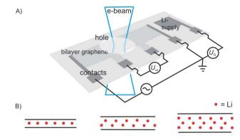
Fig. 1 Illustration of in situ transmission electron microscopy of the Liintercalation process in suspended 2L graphene, triggered in a device. (A) Illustration of the device on a Si<sub>3</sub>N<sub>4</sub>-covered Si substrate. (B) from left to right: side-views of expected 'conventional' C<sub>6</sub>LiC<sub>6</sub> configuration and of the experiment matching structures with 2L Li crystal and 3L Li crystal.15
