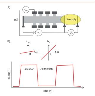
Fig. 23 (A) Illustration the 2L graphene device for measurement of Liion diffusion rates. The 2L device was shaped into a Hall bar configuration. (B) Lithiation/delithiation cycles visualized by charge carrier concentration extracted from Hall measurements showing full reversibility of the intercalation cycles.93
