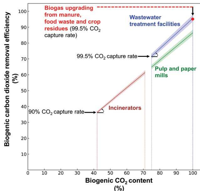
Fig. 1 Biogenic CO<sub>2</sub> content and biogenic carbon dioxide removal efficiencies from different BECCS technology chains. Solid lines represent the average scenario of CO<sub>2</sub> losses in transport and injection; shaded areas show the estimated range of CO<sub>2</sub> losses during transport and injection. Depending on the amount of biomass co-fired, biogenic CO<sub>2</sub> content in biomass co-fired power plants can vary from 1% to 100%.
