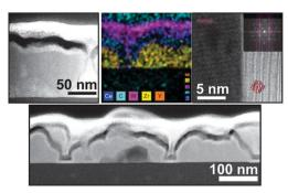
Fig. 29 TEM images and mapping results showing the epitaxial growth of ALD-derived ceria on porous YSZ thin films. Reprinted from ref. 312 with permission.
