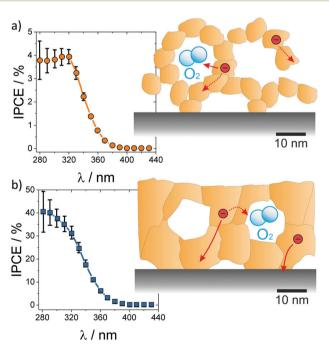
Fig. 22 Incident photon-to-current efficiency for water photoelectrocatalysis over (a) nanoparticle-derived and (b) sol-gel mesoporous TiO2 thin films. The nanoparticles in the wall structure result in low electronic conductivity and high recombination rate, while the sol-gel films with thicker and continuous pore walls reveal high photocurrents with a relatively lower recombination rate. Adapted from ref. 20 with permission.
