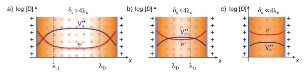
Fig. 7 Defect concentration for different grain sizes (schematically shown for  $CeO_2$ ). (a) The space-charge region affects the defect concentration near the interface in microcrystalline material. (b) For grain sizes smaller than four times the Debye length, the space-charge region starts to overlap and (c) finally completely dominates the defect concentration of the whole grain. Adapted from ref. 78 with permission.
