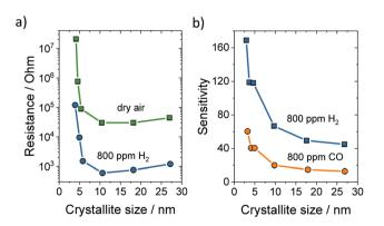
Fig. 25 (a) Electrical resistance at 300 °C in dry air or 800 ppm H<sub>2</sub> versus the crystallite size of  $SnO_2$ . (b) Sensitivity to 800 ppm  $H_2$  or CO versus the crystallite size of SnO<sub>2</sub>. Adapted from ref. 263 with permission
