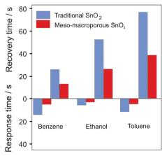
Fig. 26 Comparison of recovery and response times to 100 ppm benzene, ethanol or toluene for "traditional" SnO2 and mesoporous-macroporous SnO<sub>2</sub>. Adapted from ref. 268 with permission.
