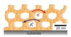
Fig. 4 Schematic illustration of the 3-dimensional architecture of mesoporous oxide thin films with efficient transport pathways for electrons and ions and a vast number of interfaces.
