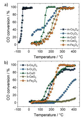
Fig. 19 CO conversion on (a) mesoporous and (b) bulk oxide catalysts. Adapted from ref. 227 with permission.
