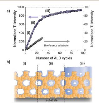
Fig. 28 (a) In situ XRF monitoring of filling of mesoporous thin films with an initial pore size of 4 nm during ALD of TiO2. After pore filling, the growth rate decreases and TiO2 only grows as a top layer on the films. (b) Schematic illustration of the pore filling process. Adapted from ref. 304
