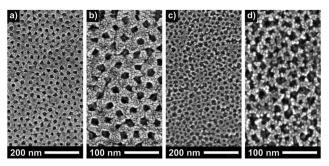
Fig. 3 Top-view SEM images of sol-gel-derived (a and b) and preformed nanoparticle-based (c and d) mesoporous  $TiO_2$  thin films. Reproduced from ref. 20 with permission.
