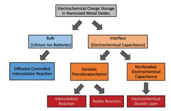
**Fig. 15** Charge-storage mechanisms in nanocrystalline metal oxides. Adapted from ref. 156 with permission.
