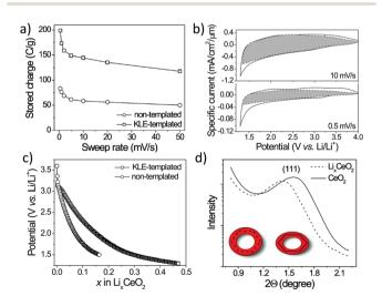
Fig. 17 (a) Charge-storage dependence on sweep rate for nanocrystalline (nontemplated) and mesoporous (KLE-templated) CeO2 thin films. (b) CV curves for mesoporous CeO2. The capacitive current is highlighted in gray. (c) Galvanostatic discharge curves at C/2 rate. (d) SAXS patterns for mesoporous CeO<sub>2</sub> and Li<sub>x</sub>CeO<sub>2</sub>. Adapted from ref. 165 with permission.
