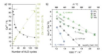
Fig. 30 (a)  $Ce^{3+}$  content of ceria deposited onto mesoporous  $ZrO_2$  thin films as function of the ALD cycle number. The  $Ce^{3+}$  content decreases with increasing coating thickness. (b) Temperature-dependence of total conductivity for mesoporous  $ZrO_2$  and  $CeO_2-ZrO_2$  composite thin films (25, 75 and 150 ALD cycles). Adapted from ref. 318 with permission.
