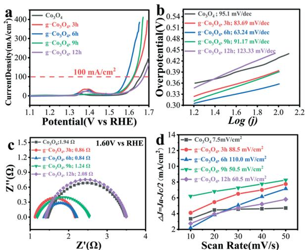
**Fig. 4** (a) LSV curves of pristine  $\text{Co}_3\text{O}_4$  (black) and  $\text{g-Co}_3\text{O}_4$  with different hydrothermal reaction times: (red) 3 h; (blue) 6 h; (green) 9 h and (purple) 12 h. (b) Related Tafel slope. (c) and (d) Nyquist plots and double layer capacitance of the as-prepared catalysts.
