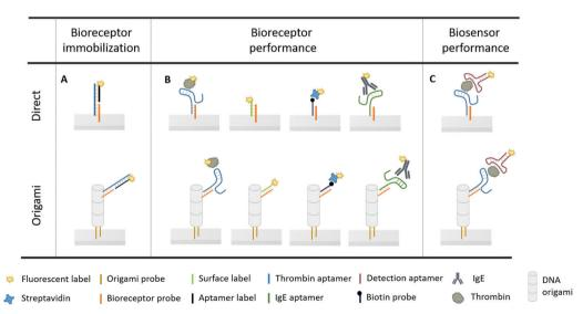
Fig. 1 Schematic overview of the different assay configurations used to test the bioreceptor immobilization, bioreceptor performance and biosensor performance. For each configuration, direct bioreceptor immobilization is compared to origami-based bioreceptor immobilization (components not to scale)
